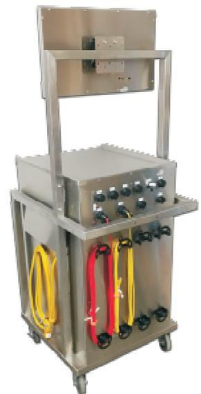
One HDMI, three USB, four RJ45 camera ports and one LAN connection are available on the carts rear panel. All ports are IP 67 rated.
